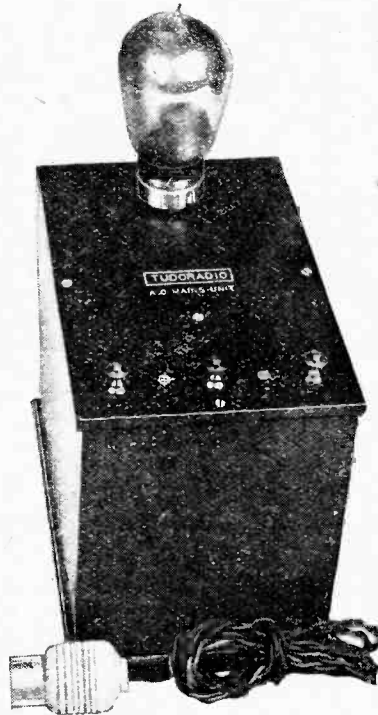
Tudoradio A.C. unit for deriving H.T. supply from A.C. mains.
