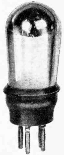
D.E.2, L.F. Nominal rating, filament, 2 volts, 0.12 ampere; anode volts 80, maximum; amplification factor, 7; anode impedance, 22,000 ohms.
