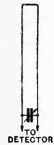
Fig. 7.—Vertical loop aerial used to demonstrate the existence of the magnetic component of arriving waves in the screen (Fig. 6).
