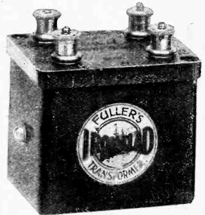
Sparta Intervalve transformer. The magnetic circuit is closed through the cast-iron screening box.
