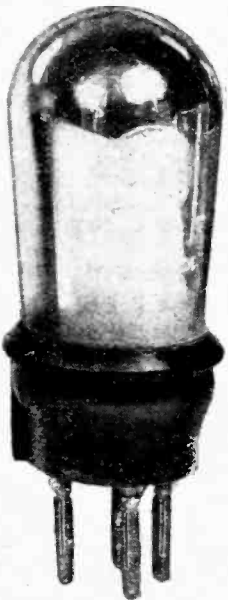
D.E.2, H.F. Nominal rating, filament, 2 volts, 0.12 ampere; anode volts 120, maximum; amplification factor, 12; anode impedance, 45,000 ohms.
